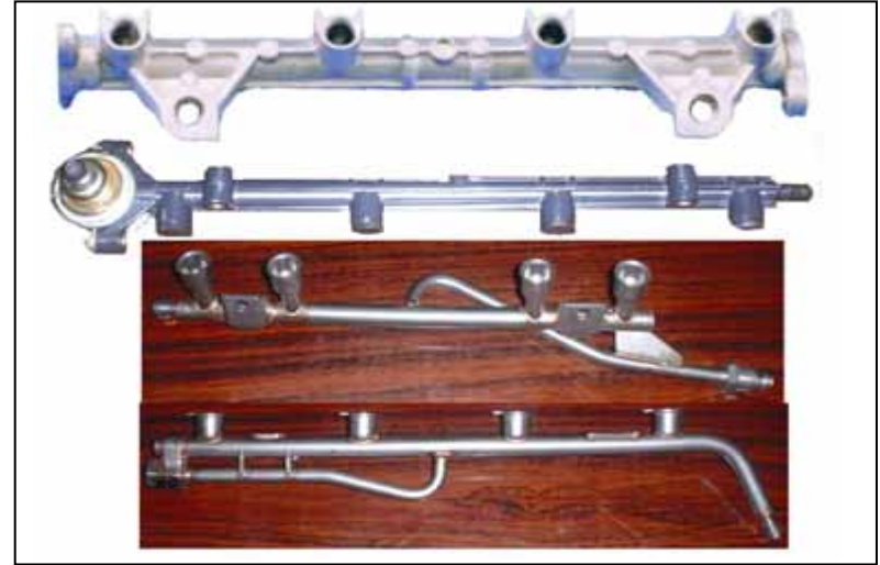
Fuel rail Manifolds.
